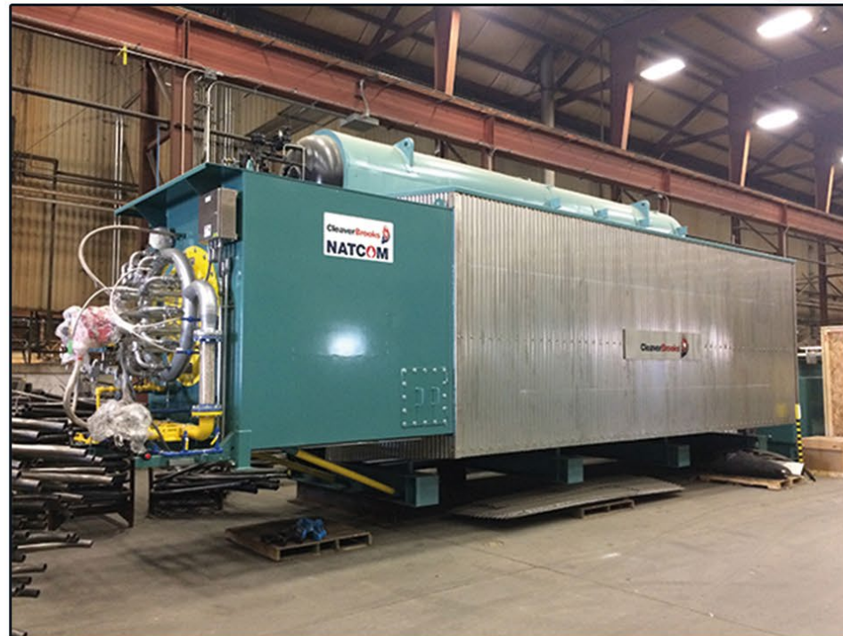
Caldera 40 ton/h Minera
